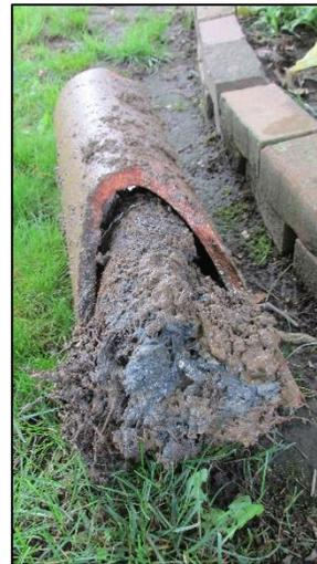
This photo is of a section of a sanitary sewer service line that was removed at a Bremen residence last year because it had become completely blocked with roots and sediment. This exemplifies the type of situation that Columbia Gas encountered at many residences in town.
